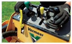
**EFFICIENCY AND PRODUCTIVITY ARE NOW MADE EASY** with a single pilot-operated ground drive joystick, which allows for a smooth range of motion. Additionally, a conveniently placed auxiliary lever by the loader arm controls, allows operators to multitask.
